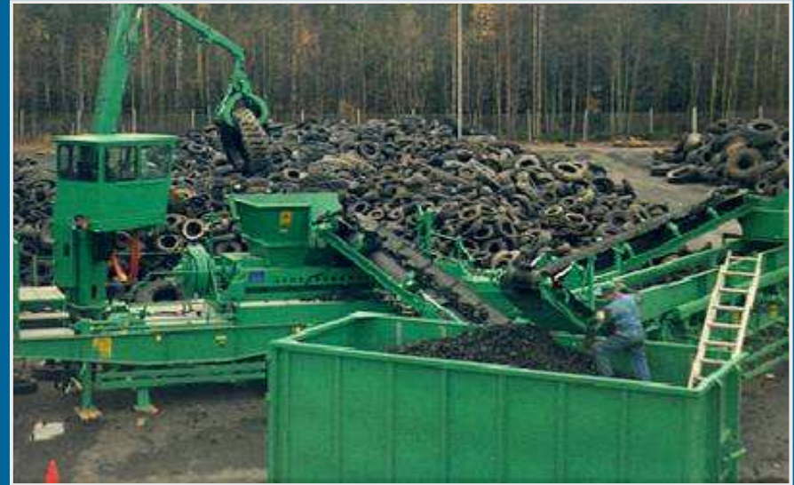
Mobile Tire Shred Mill and TDA Type B Product
